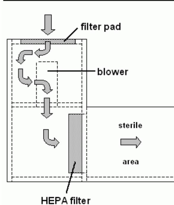
A laminar flow hood consists of a filter pad, a fan and a HEPA (High Efficiency Particulates Air) filter. The fan sucks the air through the filter pad where dust is trapped. After that the prefiltered air has to pass the HEPA filter where contaminating fungi, bacteria, dust etc are removed. Now the sterile air flows into the working (flasking) area where you can do all your flasking work without risk of contamination.
