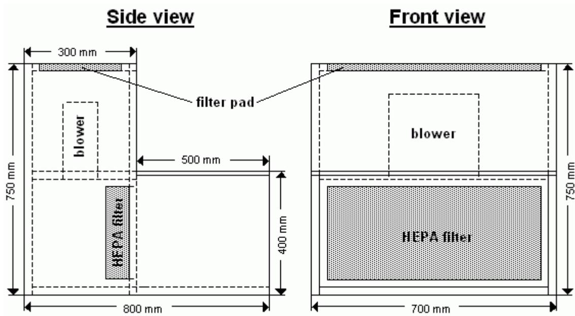
Side view of the laminar flow hood with open filter unit
